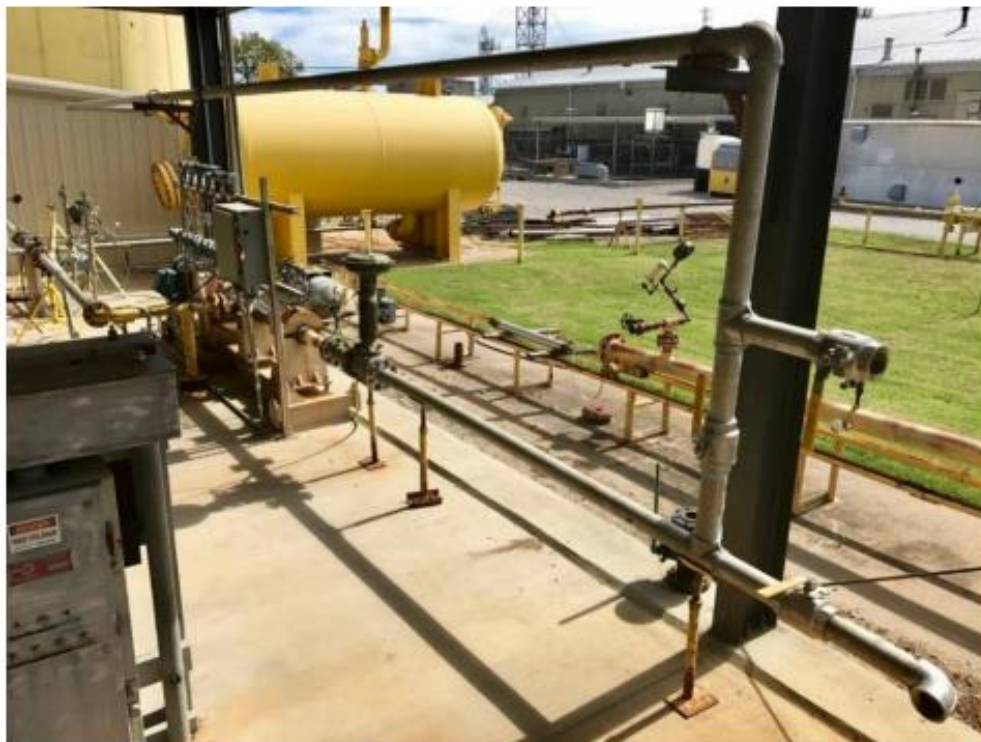
Figure 2.2 TUALP Gas-Liquid ESP Flow Loop
