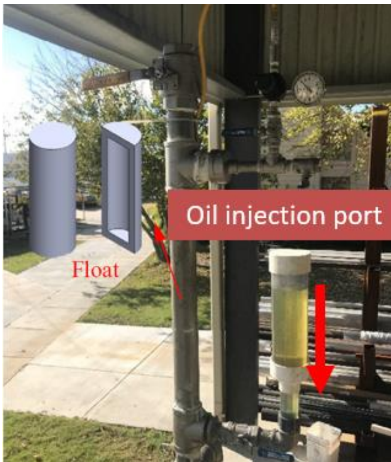
Figure A.2 Oil Injection Port
