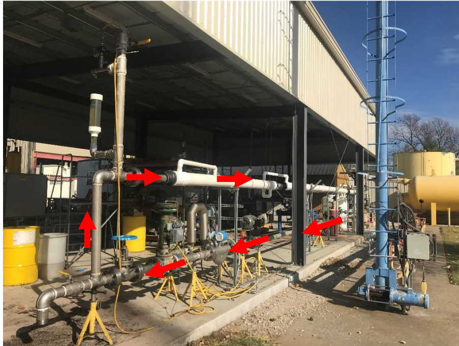
Figure 2.3 TUALP High-Viscosity ESP Flow Loop
