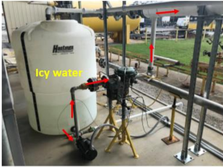
Figure A.9 Cooling System
